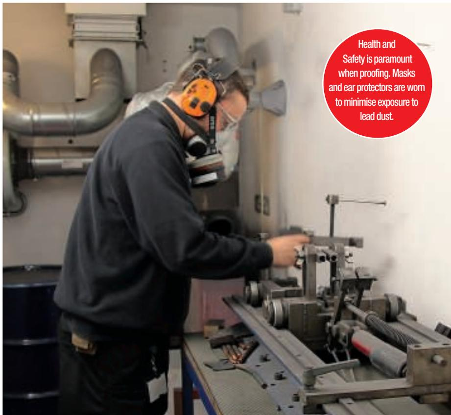
Health and Safety is paramount when proofing. Masks and ear protectors are worn to minimise exposure to lead dust.
