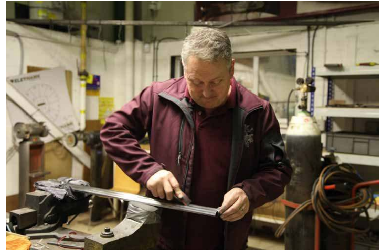
All the barrels for Longthorne shotguns are polished by hand
