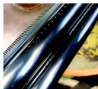
The test gun showed ported barrels. Note how the barrel set's construction enables the sighting rib to be at once solid (as befits a game gun), broad, and light
