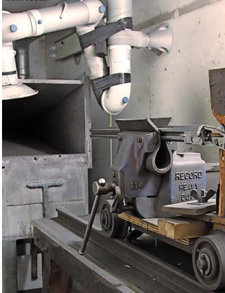
The antiquated firing machine is activated by pulling a string that is threaded through the wall into the next room
