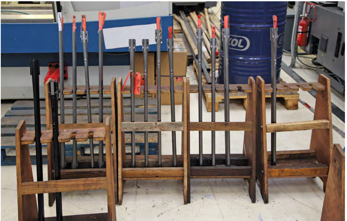
Longthorne barrels in progress (above) and almost ready for proof (below). Longthorne manufactures its barrels from a solid block of steel, including the monoblock which enables them to produce perfectly straight barrels without the distortion and metal-softening problems of many conventionally fabricated barrels.
